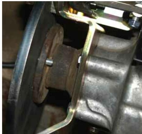
This is the correct, Long type fitted to Samurai transfer box rear outputs.
