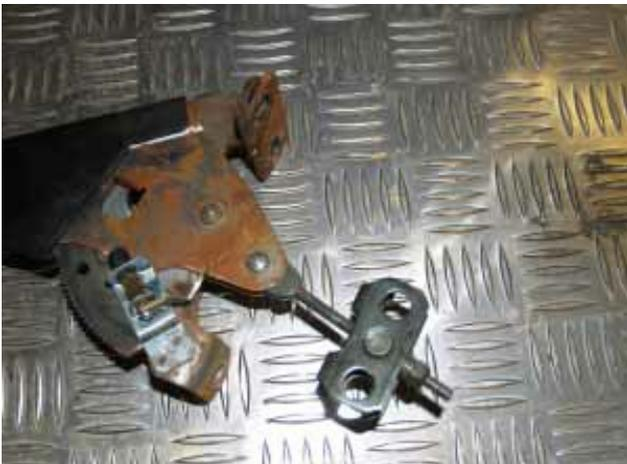
Remove your handbrake lever. If it is a dual cable type, it will look something like this. You will need to remove the toggle by grinding off the rivet which attaches it to the lever.
