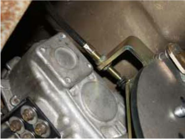
Initially set the adjustment nuts so there is plenty of scope for tightening the cable later.
