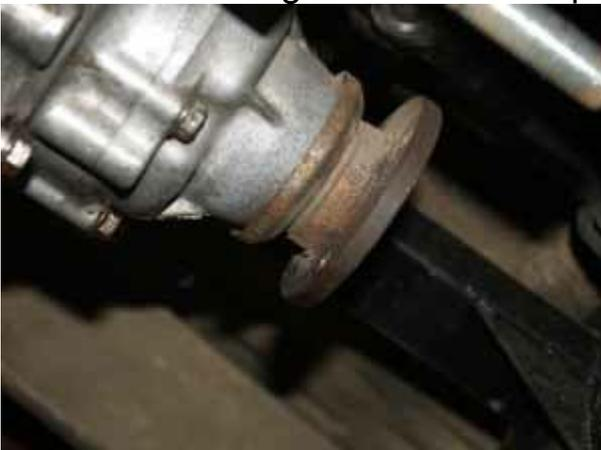
The short type above are used on the front of the transfer box as well as on the differentials. In your kit, you will find 5 big washers which can be used as a spacer. Place up to 5 washers between the bearing and the drive flange.
