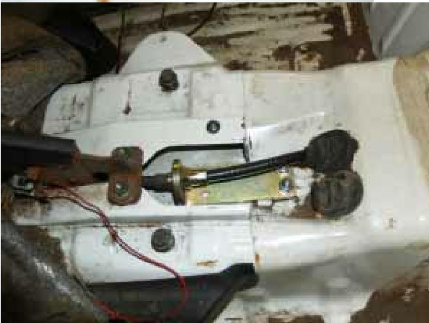
Finally adjust your handbrake such that as the disk rotates, it is only just brushed by the pads. The lever should only start to become stiff at about three clicks. Any less and your pads will wear out double quick! Once you have re-fitted your prop shafts you are ready to roll!
