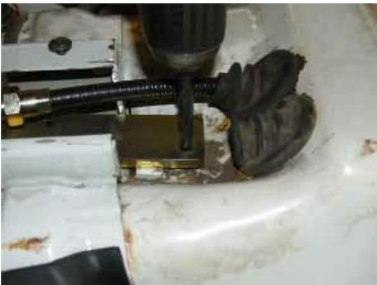
Use a grinder to make enough space behind the handbrake cable to fit the angle bracket as shown.
