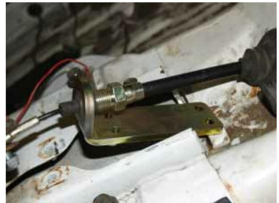
Attach the lever to the end of the cable and hold in it's proper position with the lever released. Pull the angle bracket back away from the lever. When this cable is taught, this is where to drill holes to attach the bracket to the transmission tunnel.
