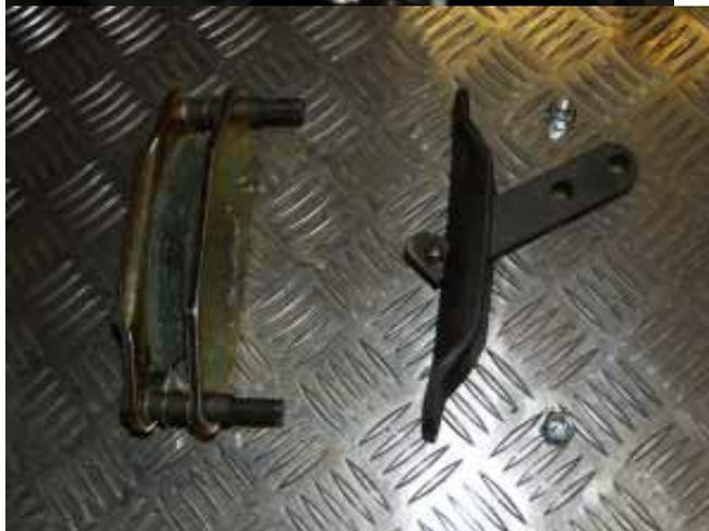
It is easiest to install the disk & caliper as one unit. Hold the parts together as shown and insert caliper bolts through receiving holes in caliper. Be careful the spacer tubes & springs do not fall out of the caliper.
