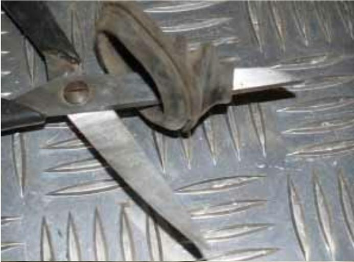
The old cables pass through the transmission tunnel wall with rubber grommets. These will not fit over the new cable, but by cutting as shown, they can be re-used.
