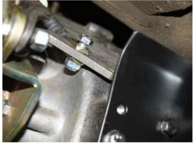
Attach the clevis on the end of the cable to the inner-most hole on the operating lever with the M8 Bolt.
