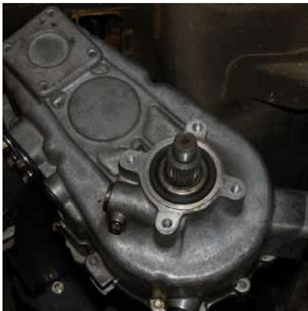
Attach the back plate to the rear of the transfer box re-using the original mounting bolts and washers. These are M8 size, just in case you loose one!
