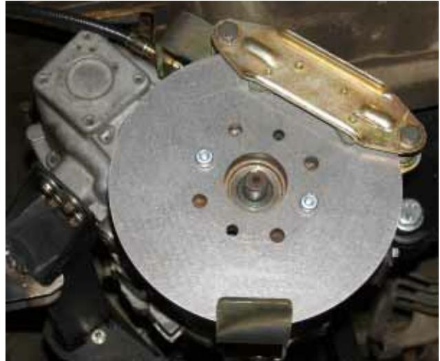
Use a couple of prop-shaft bolts to loosely hold the disk in place on the drive flange.
