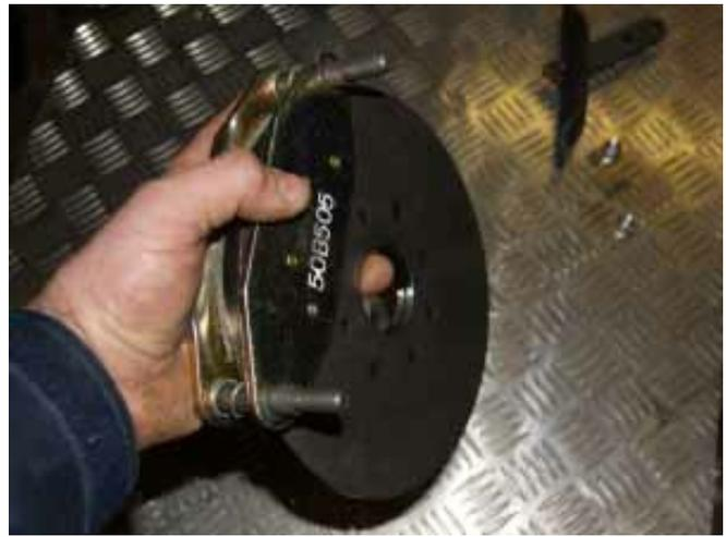
Re-assemble the caliper in-situ as shown below. Make sure the caliper operating lever is oriented such that pulling the cable will engage the caliper.
